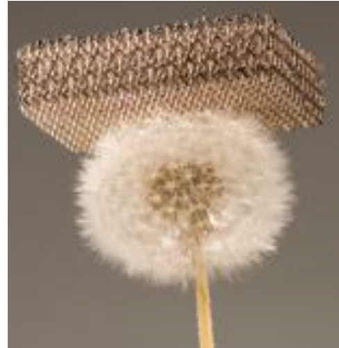
Fig. 1. An example of a 3D lattice structure, designed and fabricated by Hughes Research Labs (HRL), representing the new frontiers for materials and design. 99.99% of this metallic truss structure is air. The remaining 0.01% is made of very thin (nanometer, micron and millimeter scale) features.
