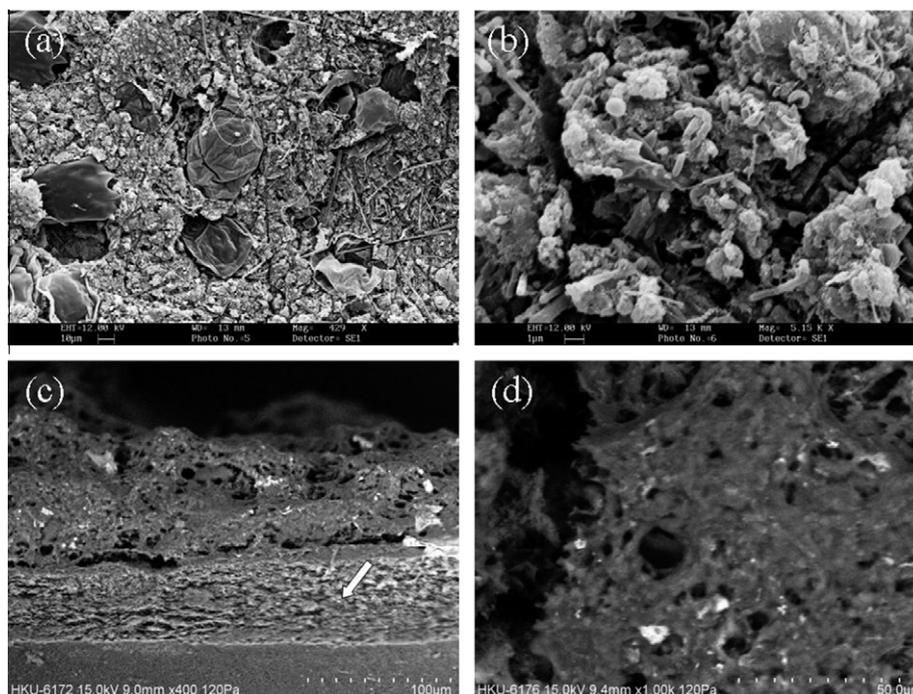
**Fig. 1.** Micrographs of the activated sludge cake layer obtained (a and b) with a conventional SEM after sample pretreatment involving dehydration and sputter coating and (c and d) with an ESEM at room temperature without prior flash freezing. The arrow points to the membrane filter.
