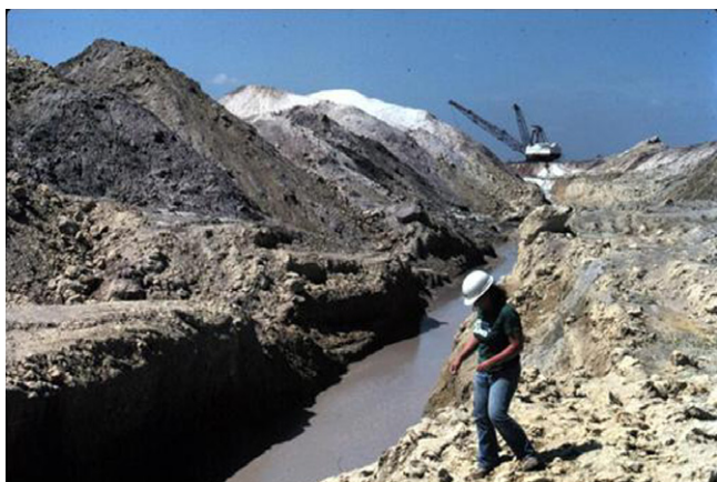
Fig. 1. Dragline mining of phosphate ore in Florida.
