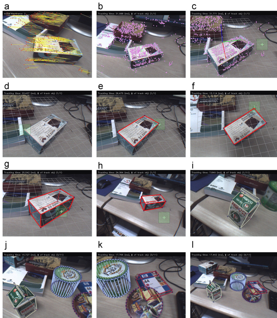
Fig. 1. Overview of the proposed approach. (a) Our system continuously reconstructs the environment and tracks the camera from the video stream. (b and c) The user can set a local coordinates upon the object surface by clicking once. (d and e) Then, the user can add control points at each corner of the video of the object to define one facet. (f) The control points can be adjusted from another point of view. (g) If the object geometry is a prism, its 3D model can be quickly obtained by extending the facet to a 3D volume. Then, (h) the object can be tracked independently. (i–l) Multiple object tracking. Various types of 3D objects are modeled and tracked very fast.
