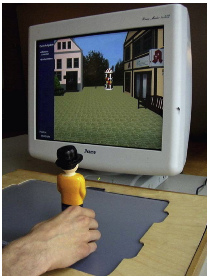
Fig. 1. User navigating through the virtual environment by moving a puppet-shaped prop over the board. Actions are initiated by pressing a button in the hat of the prop.
