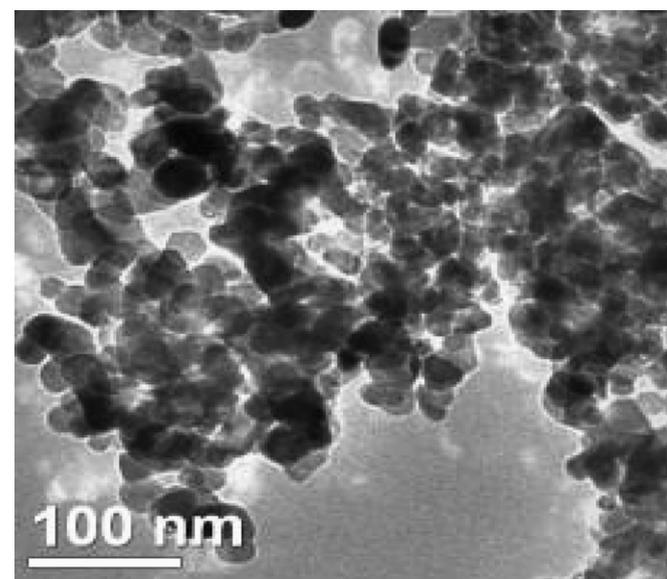
Fig. 1. TEM image of nano-ZnO sample (scale: 100 nm).
