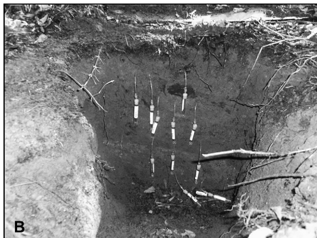
Fig. 1. Leaching column set up in the laboratory (A) and rhizon pore water samplers in the soil profile in the field (B).
