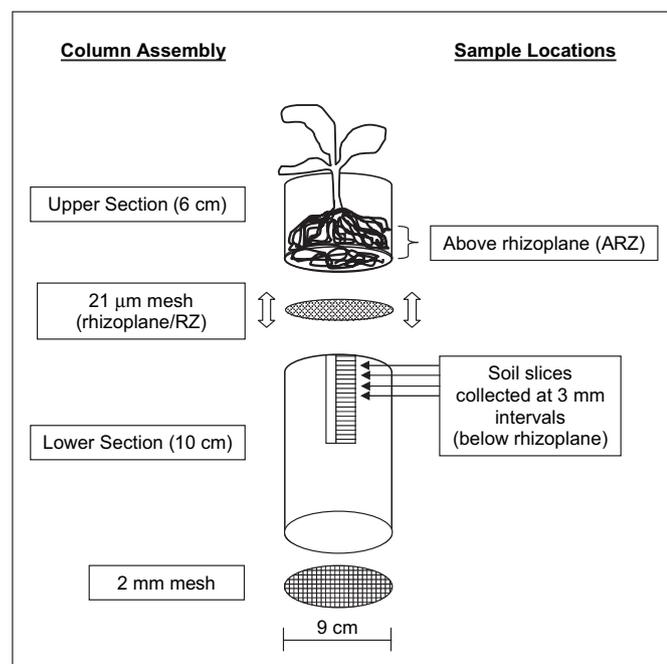
Fig. 1. Column apparatus for *Rumex crispus* experiment showing column components on the left and sampling locations on the right.
