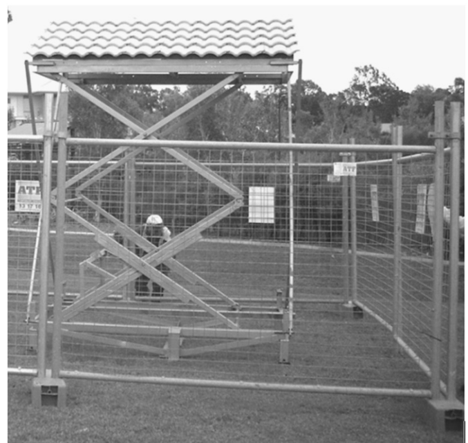
Fig. 1. A model roof used for pollutant build-up data collection.
