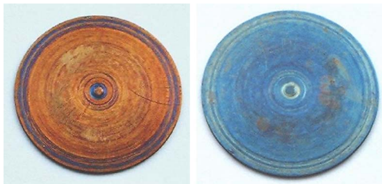
Fig. 1. Pristine DU sample (left) and the same sample after 182 days in contact with Ca-phosphate solution.
