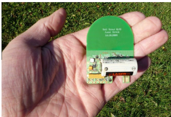
Fig. 1. Soil Scout v2 prototype with size 48 \times 68 \times 20 mm without moisture sensors. Foto: J. Tiisanen.
