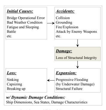
Fig. 1 Structural links of damage scenarios.
