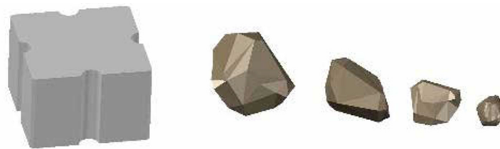
Fig. 1 Virtual 3D models of stones and antifer.
