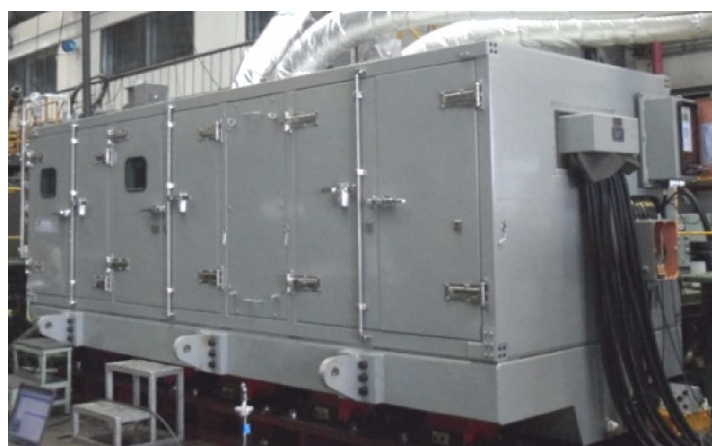
Fig. 1 An example of large acoustical enclosures for marine diesel generators.
