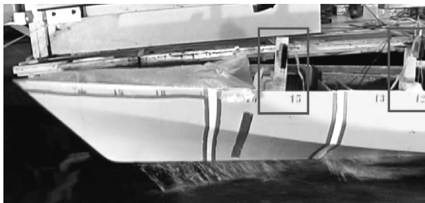
Fig. 2 Side view of the physical model at the end of water-exit phase and wire-probe positions.
