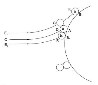
**Fig. 1.** Shadowing effect and chain-like deposition. Figure based on Wang (2001).
