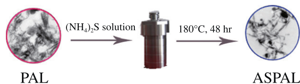
Scheme 1 – Schematic diagram of the hydrothermal activation process. PAL: palygorskite. ASPAL: PAL modified with ammonium sulfide.
