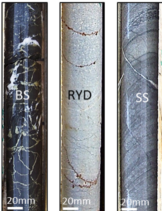
Fig. 2. Representative photographs of classes used for lithofacies modeling; abbreviation BS = Black shale RYD = Rhyodacite SS = Sandstone.
