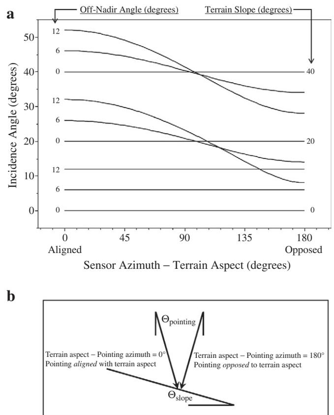
Fig. 1. A) Evaluation of the local incidence angle equation to illustrate the combined effects of terrain slope, off-nadir pointing and the angle between terrain aspect and sensor point angle. B) Illustration of the angle between terrain aspect and sensor point angle.
