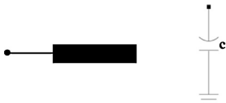
Fig. 3. Layout and equivalent LC circuit of open-end.
