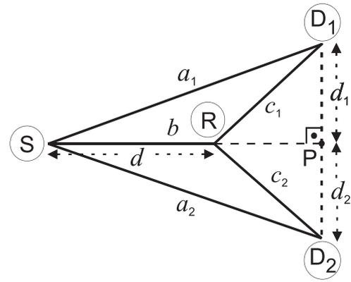
**Fig. 1.** The broadcast relay channel (BRC), with one source (S), one relay (R), and two destinations ( $D_1, D_2$ ). For the numerical simulations in Section 4, all four nodes are located on a plane with  $S$ - $R$ ,  $D_1$ -point  $P$  and  $D_2$ -point  $P$  distances are respectively equal to  $d, d_1$  and  $d_2$ .
