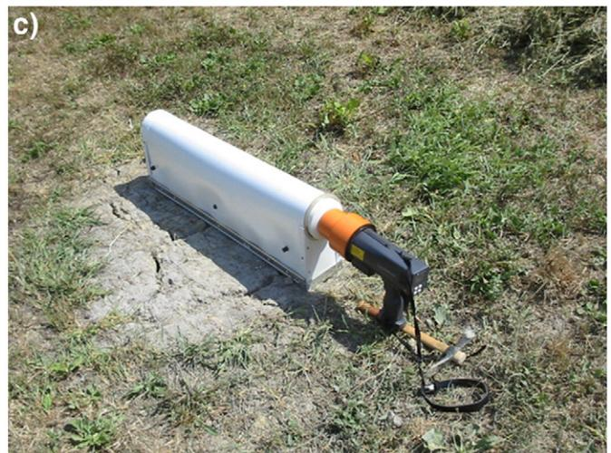
Fig. 2. Photos of the closed-chamber systems used in microseepage surveys in USA (a) and Europe (b, c). Methane concentration increase is measured by GC analysis of samples taken manually by syringes (a, b) or by direct detection by laser sensor (c).
