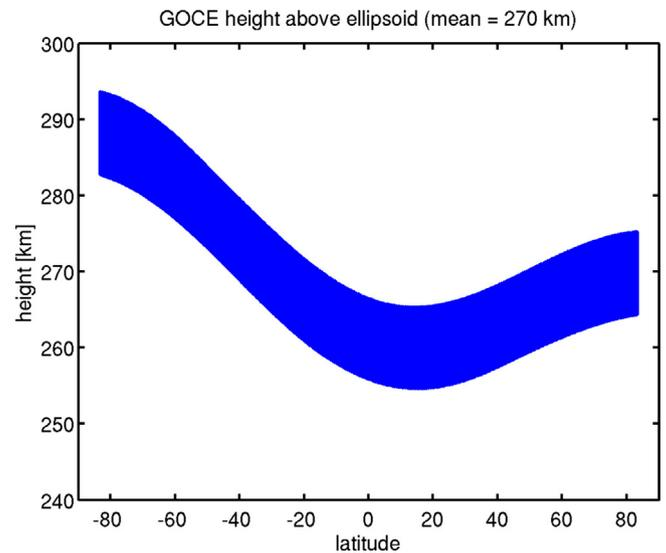
Fig. 1. Height of the GOCE satellite above the ellipsoid as a function of latitude.
