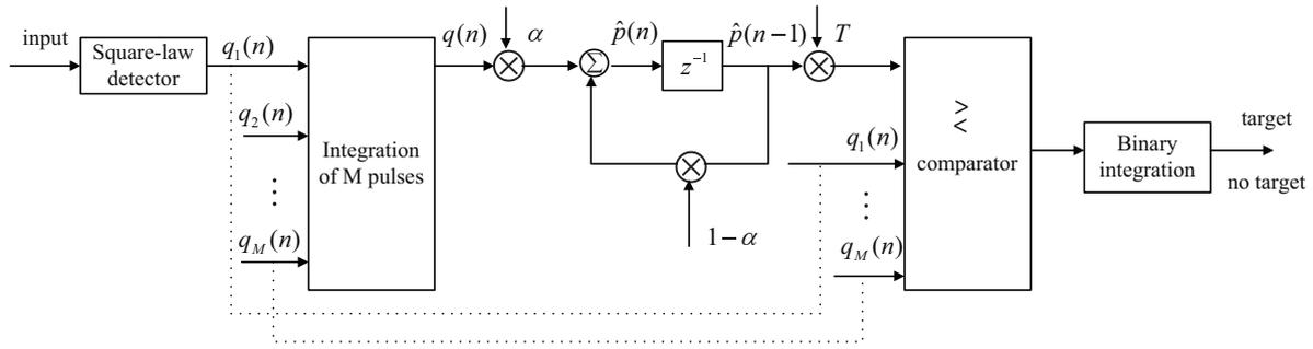
Fig. 1. The block diagram of the clutter map with binary integration.
