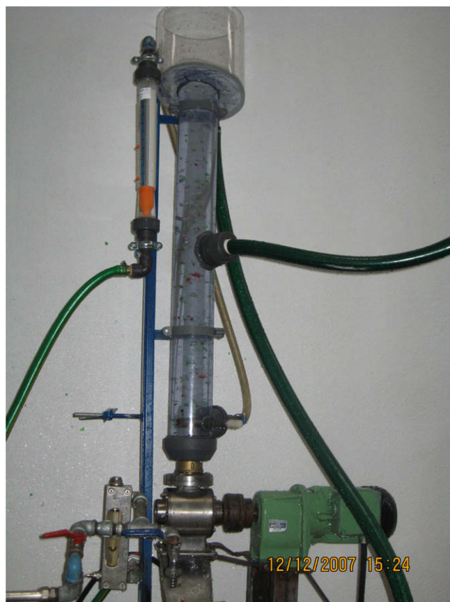
Fig. 2. The fluidized bed classifier used.
