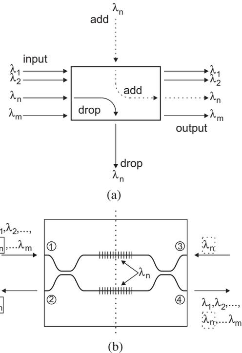
**Fig. 2.** Network function of an add/drop-multiplexer and schematic realization based on a Mach-Zehnder interferometer. The device is symmetric with respect to the dashed line.
