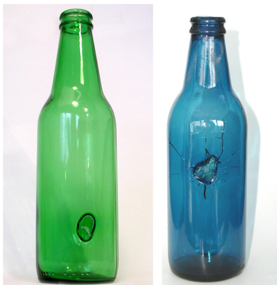
Fig. 1. Example of glass bottles showing defects due to the presence of glass-like contaminants.
