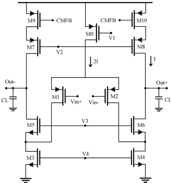
Fig. 1. Schematic of conventional folded cascode amplifier.
