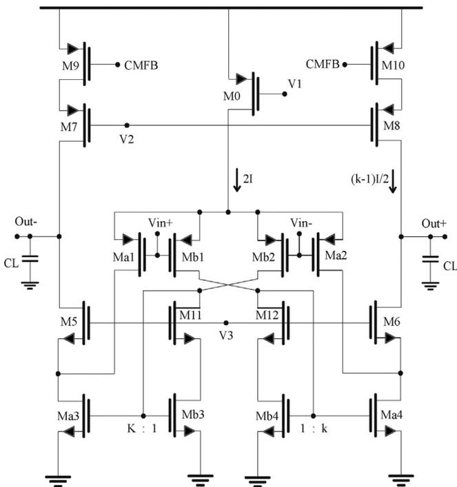
Fig. 2. Schematic of recycling folded cascode amplifier.
