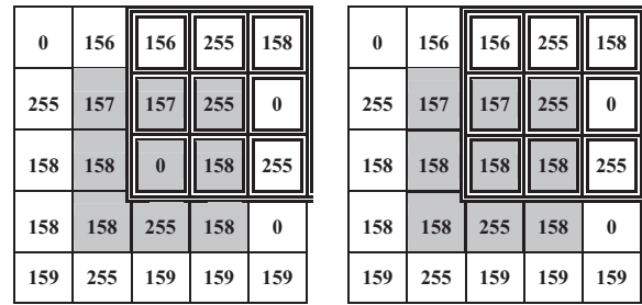
Fig. 1. (A) Two local regions before the filter and (B) Two local regions after the filter.
