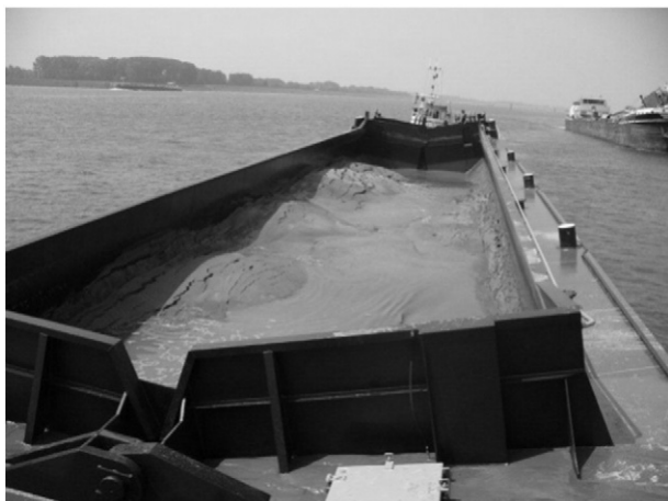
Fig. 1. Split-hull barge with Courtesy of International Marine Consultancy (IMCBrokers). Note the longitudinal hull splitting and the lowered gunwale (reduced freeboard).
