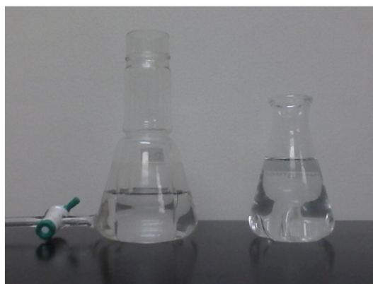
Fig. 2. Standard-size baffled flask (left) and scaled-down/low-energy baffled flask (right) employed in effectiveness tests, each filled with 120 mL synthetic seawater as they are during testing.
