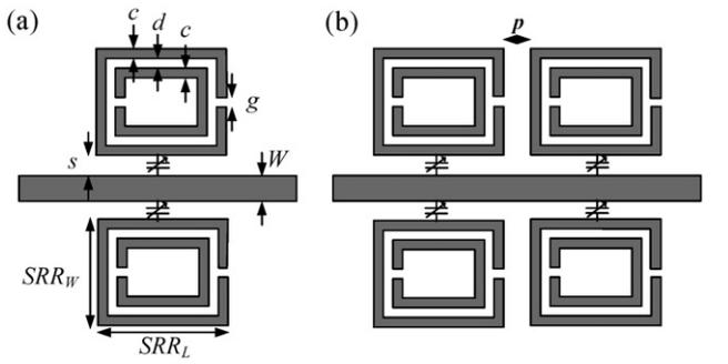
**Fig. 1.** Geometries of (a) a frequency tunable SRR stopband filter and (b) a bandwidth tunable SRR stopband filter.
