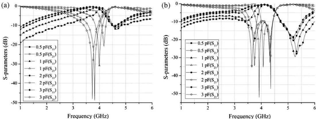
**Fig. 3.** Simulated  $S$ -parameters: (a) a frequency and (b) a bandwidth tunable SRR stopband filter with different capacitance values.
