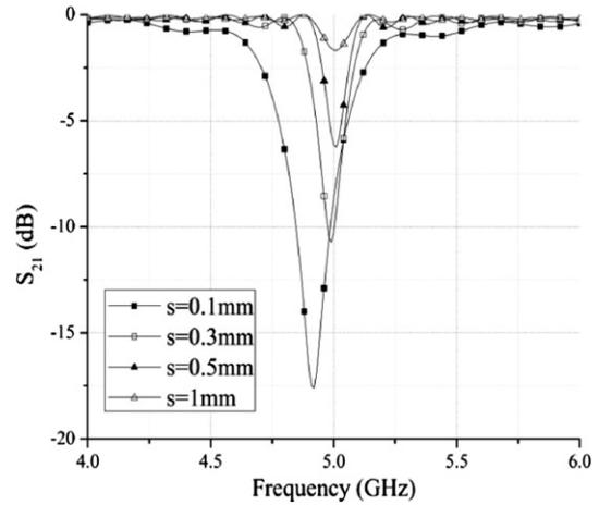
**Fig. 2.** Simulated  $S_{21}$  of a conventional SRR stopband filter as a function of  $s$ .
