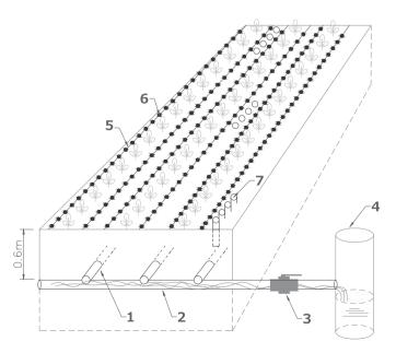
**Fig. 2.** Surface distribution system and underground drainage system. 1—Drainage pipe, 2—collecting pipe, 3—ball valve, 4—well, 5—capillary, 6—hole on the capillary, 7—soil percolation pipe.
