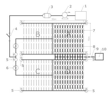
**Fig. 1.** Schematic diagram of distribution system and drainage system. 1—Anaerobic lagoon, 2—pump, 3—grit filter, 4—screen filter, 5—valve, 6—water meter and electromagnetic valve, 7—capillary, 8—drainage pipe, 9—collecting pipe, 10—well. (A) Intercropped with ryegrass with installed subsurface drainage; (B) intercropped ryegrass without installed subsurface drainage; (C) no ryegrass and no subsurface drainage; (D) no ryegrass with installed subsurface drainage.
