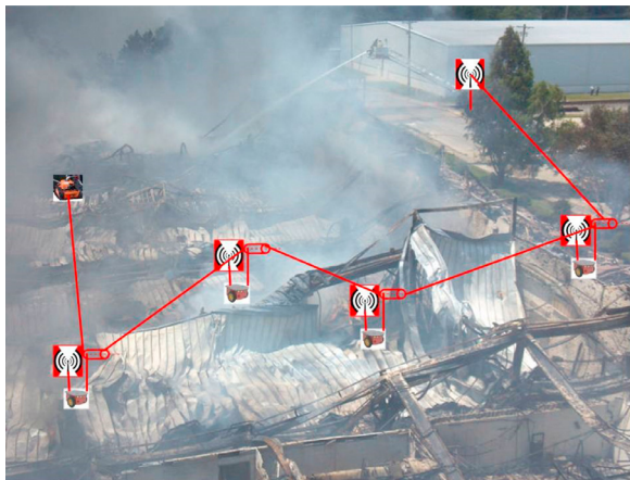
Fig. 1. A firefighter linked to command center through a set of relay robots.
