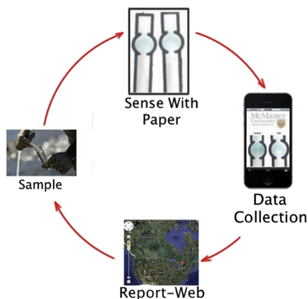
Fig. 1 – Paper-based sensors can change how water quality is tested and monitored globally. Cell phones can be used for data collection and to push data to a website where data is displayed on a map. Areas of contamination become easy to spot and can trigger additional monitoring to take place.
