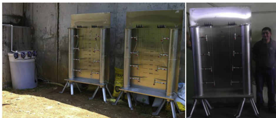
Fig. 1 – Sulfur and limestone packed pilot scale bioreactors.
