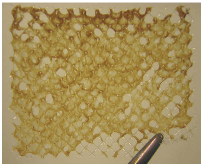
Fig. 1 – Feed spacer taken during autopsy of spiral-wound membrane module from a full-scale installation suffering from a prolonged elevated feed channel pressure drop.
