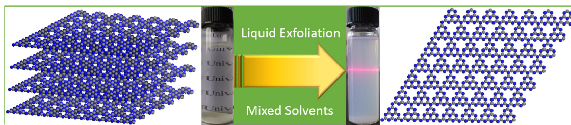
Fig. 1. Schematic illustration of mixed solvent exfoliation process from layered g\text{-C}_3\text{N}_4 powders to \text{C}_3\text{N}_4 nanosheets with molecular thickness.
