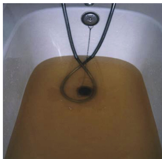
Fig. 2 – Example of discoloured water leading to customer complaints.
