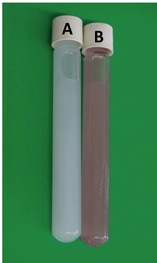
Fig. 1. Image showing the mixture before the photocatalytic process (A) and after 3 h of oxidation (B).
