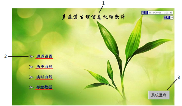
Fig. 3 – The system main interface, including the software name (pointed by line 1); channel selection, historical curve, real-time curve and data storage (from top to bottom pointed by line 2) and a reset button (pointed by line 3).
