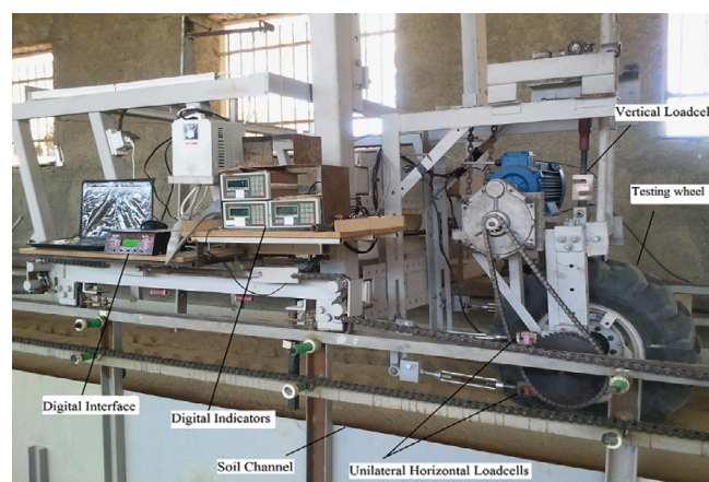
Figure 1 The general system set up of the single-wheel tester in a soil bin.
