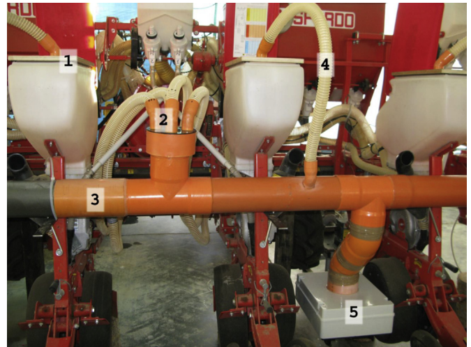
Fig. 1. The drill with the prototype device developed at CRA-ING. (1) airtight gasketed lids replacing the normal lids and provided with pipes (4) channelling the air from the main collector (3) into the hoppers. (2) collector of pipes coming from the drill's fan; (3) main pipe collector. The excess air passes through the box with filter (5) and is directed towards the ground.
