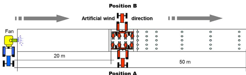
**Fig. 1.** - Scheme of the equipment disposition in the tunnel during the test.
