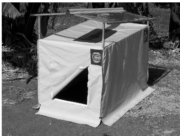
Fig. 1. Augmentorium prototype designed in Reunion Island (see the net on the top of the structure under the roof).
