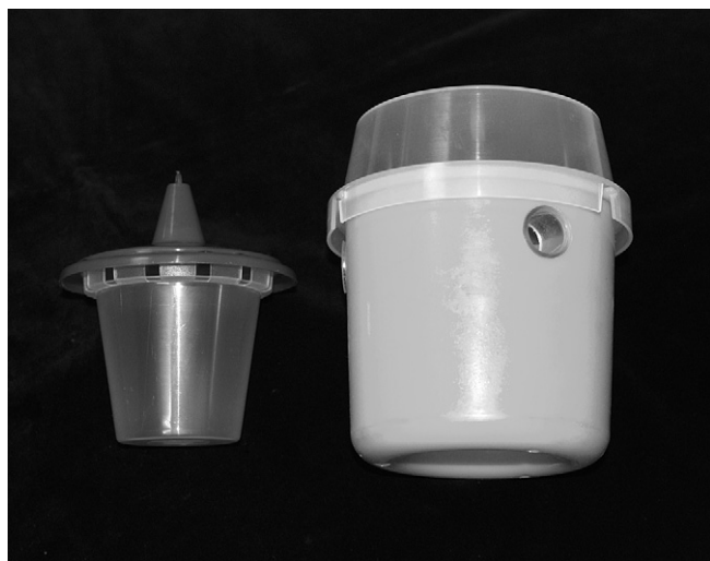
Fig. 1. The Sensus trap on the left with a royal blue lid and transparent container and the Probodelt bucket trap having a yellow container and a transparent lid.
