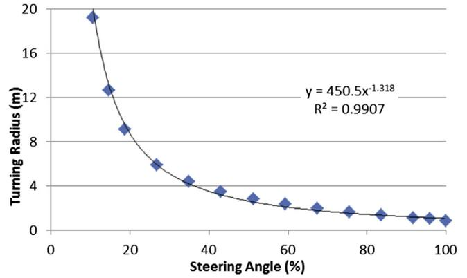
Fig. 3. Relation between turning radius and steering angle.
