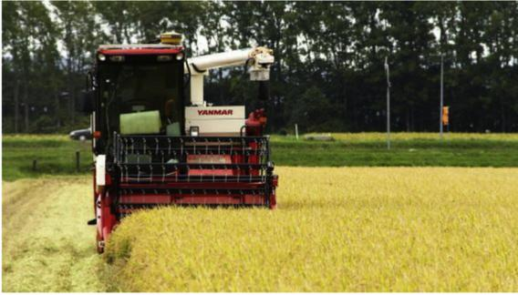
Fig. 1. The robot combine (Yanmar AG1100).
