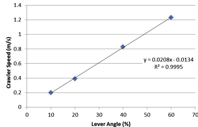
Fig. 2. Relation between speed and lever angle in straight movement.
