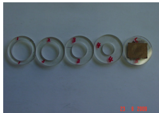
Fig. 4 Air plugs for adjustment of air velocity [L-R, No. 1 (35 mm hole), No. 2 (30 mm), No. 3 (25 mm), No. 4 (20 mm) and No. 5 (0 mm)].
