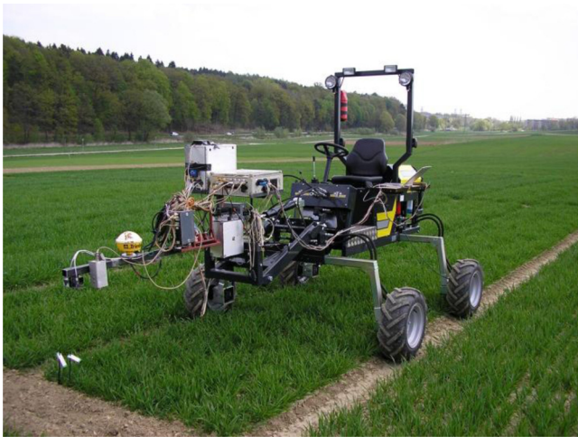
Fig. 1. PhenoTrac 4, measuring platform equipped with hyperspectral, thermal and laser distance sensors developed by the Chair of Plant Nutrition of the Technical University of Munich.
