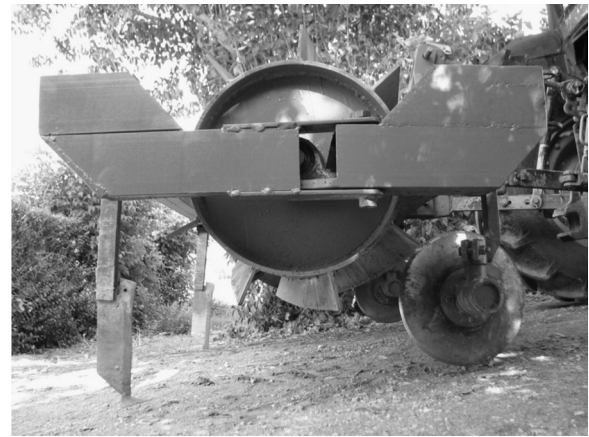
Fig. 1. Modified roller crimper for transplanting bed preparation (in-line tillage/roller crimper).
